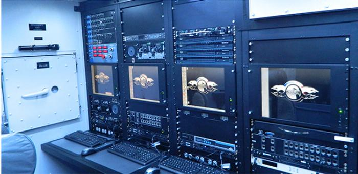
The Steel Eagle is a configurable communications module that provides advanced communications and network capabilities to the SLICC, ROCC, or other RORO systems. It provides power management, wideband (X/Ku/Ka-band) and narrowband (Inmarsat) communications, VTC, enhanced monitoring, and other capabilities.
