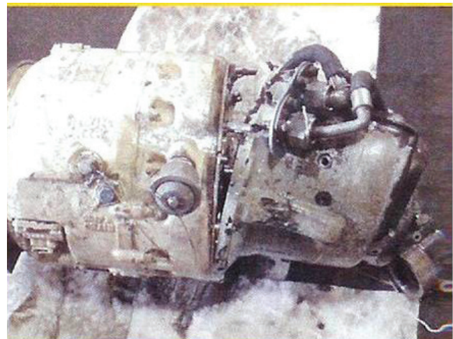
CASE OVERPRESSURE FAILURE
