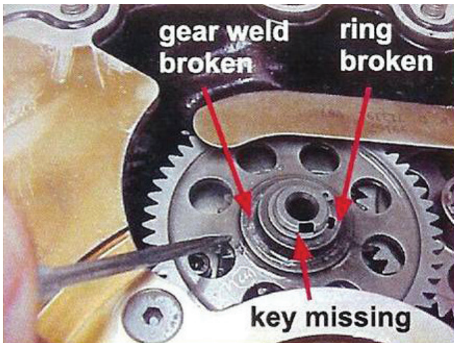
CSD PREVIOUS GEAR FAILURE
