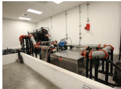
UNIVERSAL FUEL FLOW TEST STAND
