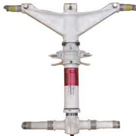
Lockheed L-100 (C-130) Nose Landing Gear
