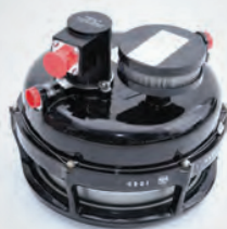
SECONDARY OUTFLOW VALVE NSN: 4820-01-312-1675 P/N: 103698-1 HONEYWELL (CAGE 64547)
