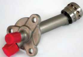
FUEL INJECTION NOZZLE NSN: N/A P/N: 3107126-1 HONEYWELL (CAGE 99193)
