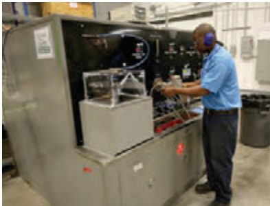
Fuel Control Test Stand
