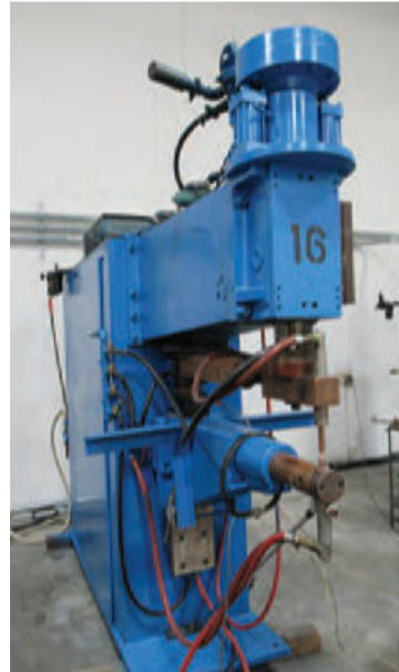
Spot Welding Machine
